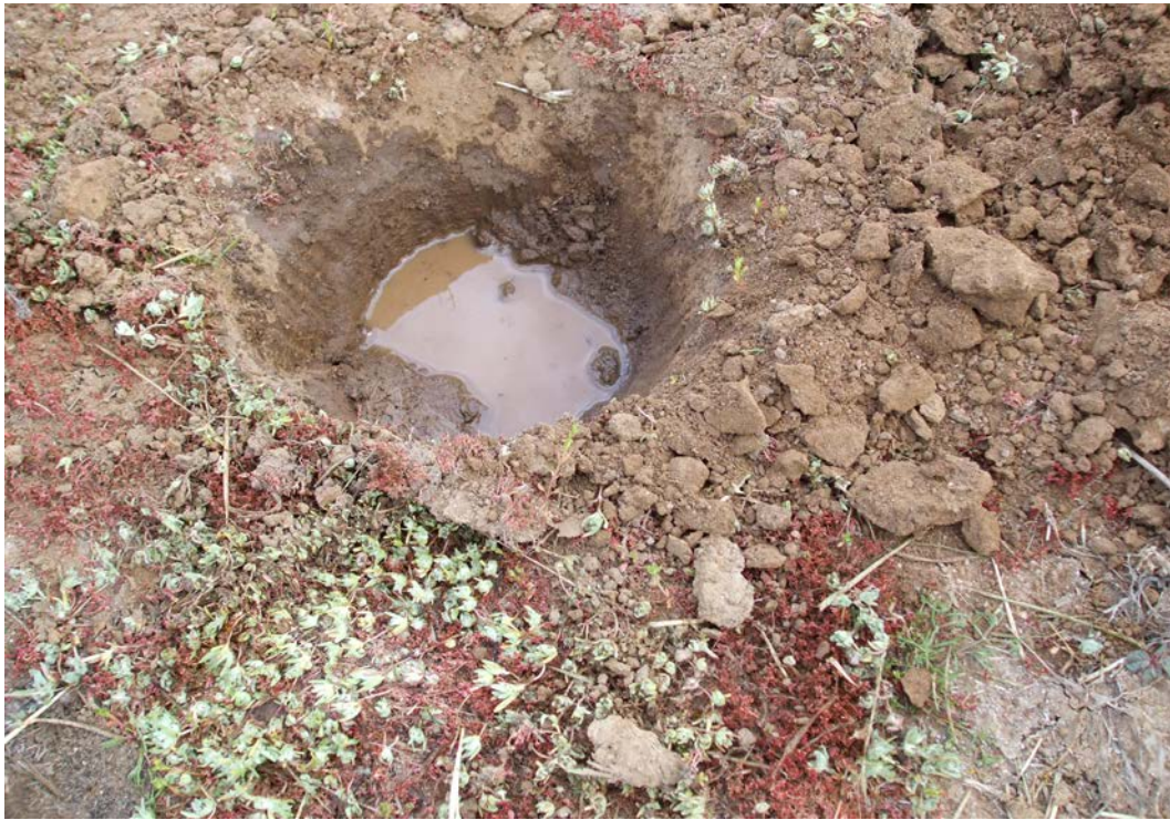
Photo 1 (April 2009): Wetland delineation soil pits were difficult to dig due to hard layer within the top few inches. Water poured into pits did not readily absorb, as depicted in the above photo.
